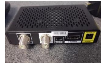
Once the coax line is attached to the "Cable In" on the back of DTA, then connect the HDMI cord to the HDMI port on the back of the DTA. One end of the HDMI cord will attach to the back of the DTA and the other end to an HDMI port on your TV.
