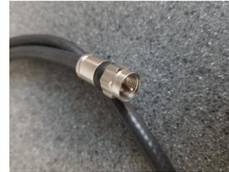
The coax line will be attached to the floor or wall outlet. Screw the end not connected to the wall/floor into the back of the DTA where it says "CABLE IN".
