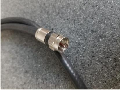
The coax line will be attached to the floor or wall outlet. Screw the end not connected to the wall/floor into the back of your tv.
